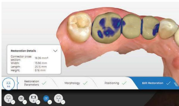
Fig. 18: Mesial connector size
