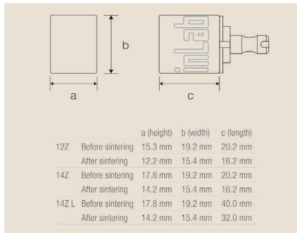
Fig. 2: Sintering effects
